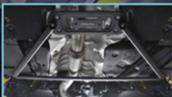
● BMW F2X/F3X 1,2,3,4 Series upgrade front strut bar & lower braces
