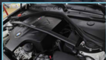
● BMW F2X/F3X 1,2,3,4 Series upgrade front strut bar & lower braces
