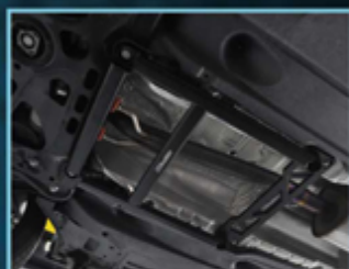
● VW Golf mk7 upgrade front & rear anti-roll & lower braces
