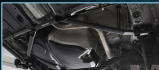
● VW Golf mk7 upgrade front & rear anti-roll & lower braces
