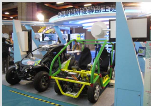
The MIRDC No. 4 open chassis platform features Space Frame structure design and high-strength steel.
