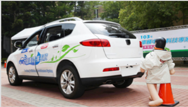
The vehicle parking collision avoidance system combines vehicle sensors, speed sensors and integrated electric parking brake (IEPB) technology to execute braking and assist with parking.
