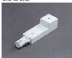
W-338 Live end conduit fitter. Designed to accept standard 3/4" trade size conduit fitter. Use when feeding to track through surface conduit system.
