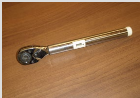
The prototype of Taiwan's first digital torque wrench was developed by ITRI.
