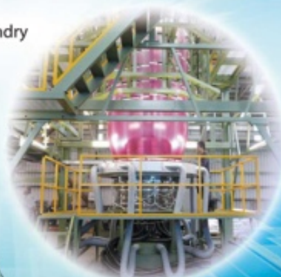
Agricultural/Industrial-duty Blown-film Extrusion Line (max. thickness: 3,000µm) 大型農業、工業用膜生產線 (最厚3,000µm)
