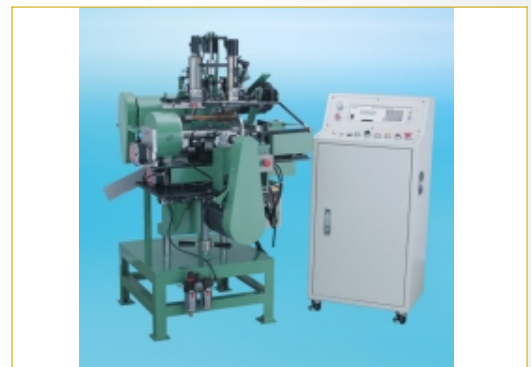
Wooden handle round comb Making Use Automatic Hole Punching and Flocking
