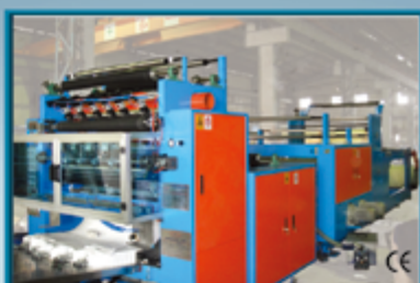
▲ V FOLD TISSUE PAPER CONVERTING MACHINE WITH MICRO TO MICRO AND GLUE SYSTEM
