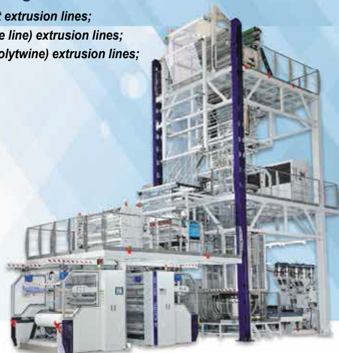
Multi-layer Co-extrusion Blown Film Extruder JC-CX Series
