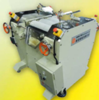
三滾筒機 Three roller mill machine
