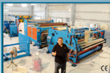
▲ REWINDER WITH POINT TO POINT AND GLUE SYSTEM FOR MAXI ROLL AND JRT ROLL
