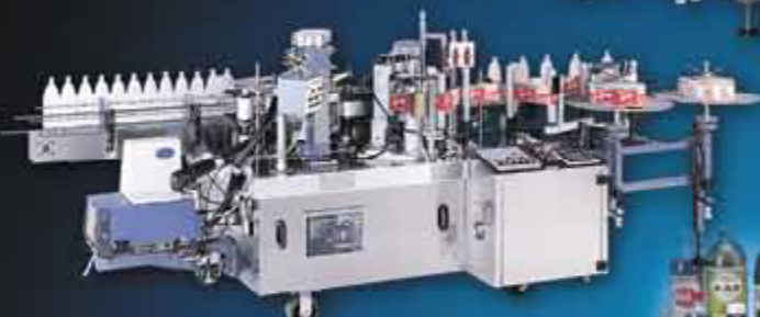
▲ MD3000-OPP 熱熔膠高速全自動圓瓶貼標機 Automatic high-speed OPP labeling machine for round bottles
