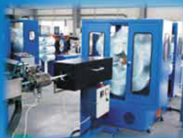
Extrusion line for flexible hoses reinforced with spiral yarn inserts 包紗軟管押出設備
