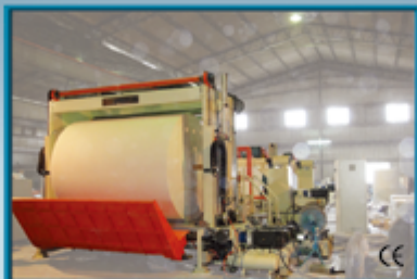
▲ SLITTING AND REWINDING MACHINE WITH FULL SERVO MOTOR
