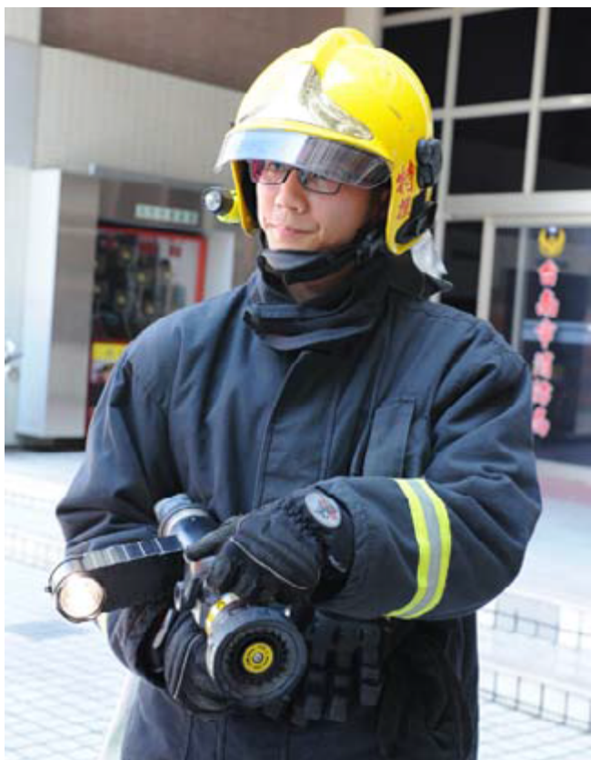
The headlamp can be mounted directly onto a firehose nozzle to enhance firefighting efficiency and safety.
