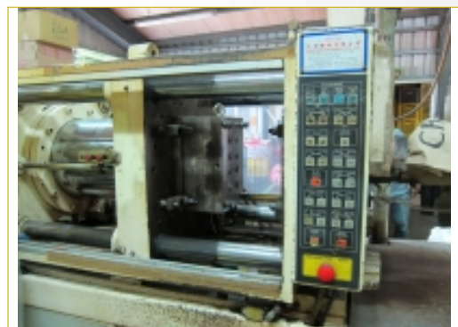
160T plastic injection molding machine
