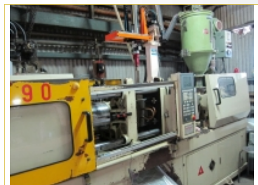
120T plastic injection molding machine
