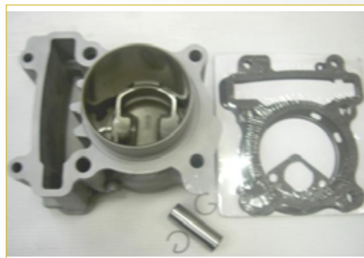
YAMAHA S-Max155 Big bore water cooler cylinder
