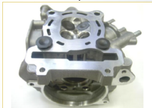
YAMAHA S-Max155 oversize cylinder head
