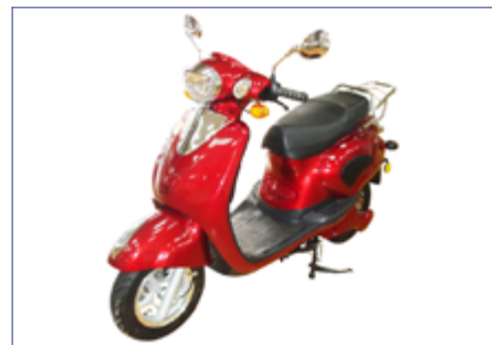
Twin 200-Motor 2000w, DC48Vx36AH Lead-Acid Battery
