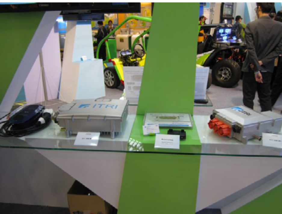
ITRI showcased a 50kW EV motor controller, the first such device developed and made in Taiwan.
