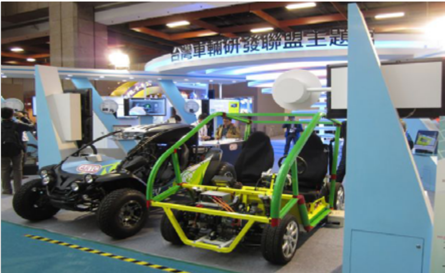
The MIRDC No. 4 open chassis platform features Space Frame structure design and high-strength steel.
