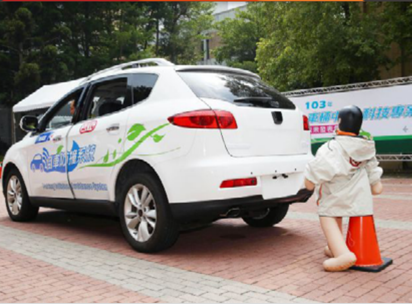
The vehicle parking collision avoidance system combines vehicle sensors, speed sensors and integrated electric parking brake (IEPB) technology to execute braking and assist with parking.
