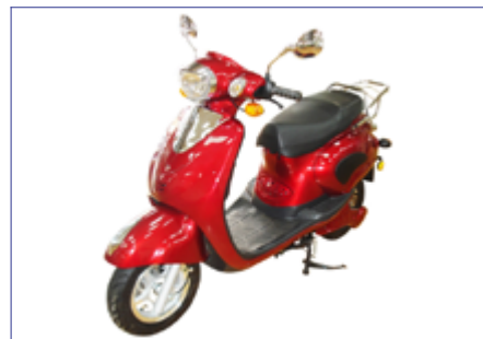
Twin 200-Motor 2000w, DC48Vx36AH Lead-Acid Battery
