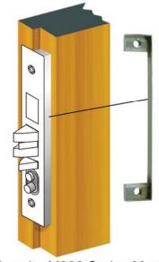
Rebate kits are essential to ensure correct closing on double doors with an overlap (rebate). Measurements are the width of the rebate.
