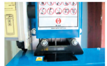
Roller fairlead for the steel cable
