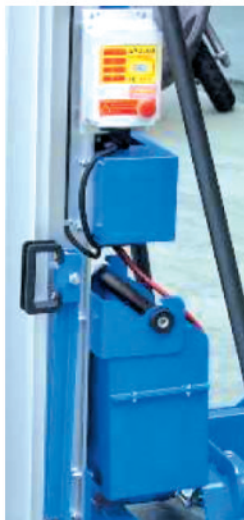
Cable under steel crankbase and crane lifting point for safe transportation.
