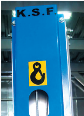
Cable under steel crankbase and crane lifting point for safe transportation.
