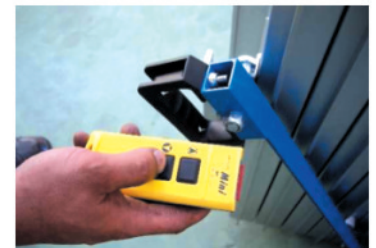
Radio remote control with emergency stop
