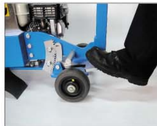
Cutting depth adjustment: variable with indication via toothed wheel.
