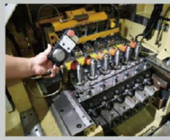
Dial Control Style Slow Jog System 手搖輪慢寸動功能
