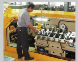
Transfer Housing Lift & Turn System 夾仔台旋出機構
