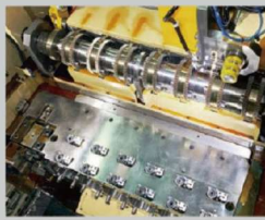
Finger Open / Close Cam Auto. Adj. 夾仔開啟凸線電動調整
