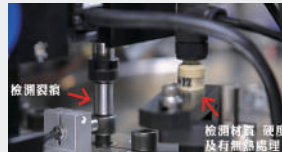
360° head side crack checking system by Eddy Current
