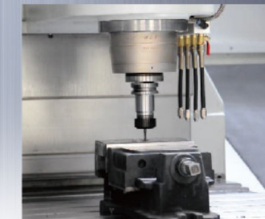
Rigid tapping test • It is necessary to do rigid tap test before make shipment. Tapping range : 3, 4, 5, 6mm
