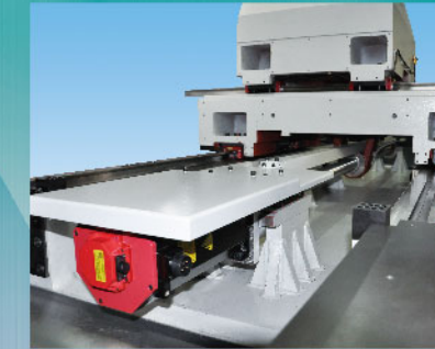
X axis ball screw • X axis ball screw assembly is with protected chip cover.
